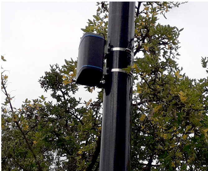
Figure 2: Zephyr® air quality sensor deployed to a lighting column in Coventry City Centre
